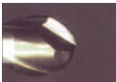
No.1 (A) cBNスパイラル刃エンドミル No.1 (A) cBN Spiral Endmill (6個加工後) (after 6pcs. Cutting)
